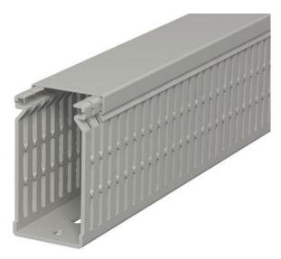
Wiring duct, incl. cover and base perforation, for horizontal and vertical routing of electrical cables in the switchgear cabinet. Designed as a metric duct. The nominal dimension of the system size corresponds to the internal dimension of the duct. Retainers are broken out without tools. The flush-floor routing of cables is possible through predetermined break points. Tapering in the side slots prevents the cables from falling out. Tested to DIN EN 50085-2-3. Special lengths on request.
